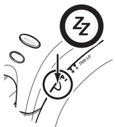
The Pebble printer may be left in stand-by at any time by pressing the push button as indicated. The green light on the push button goes out.
